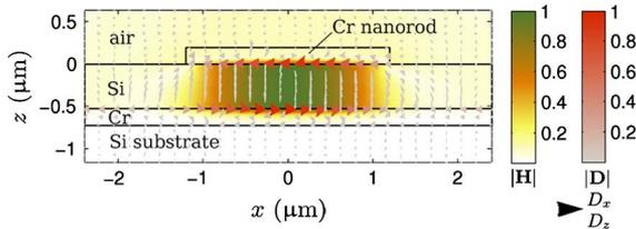
Fig. 5. Field map of the TE outgoing leaky mode in the  $Oxz$  plane for  $d = 4.8 \mu\text{m}$ . The left colormap represents the norm of the magnetic field  $H$ ; the arrows represent the direction of the displacement current  $D$ ; and their colors (right colormap) and size are proportional to its intensity.
