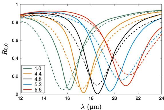
Fig. 2. Reflection spectrum at normal incidence in the specular order  $R_{0,0}$  as a function of incident wavelength  $\lambda$  for different values of the period  $d$  (in  $\mu\text{m}$ ). Solid lines, full wave FEM simulations; dashed lines, FTIR measurements.
