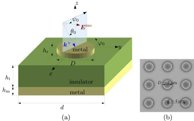
Fig. 1. Geometry of the studied structures. (a) Schematic representation and notations. (b) SEM image (top view) of a fabricated grating.
