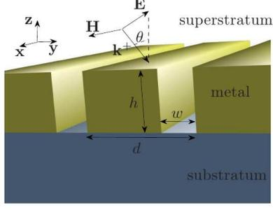
FIGURE 7. Schematic of the grating under study.
