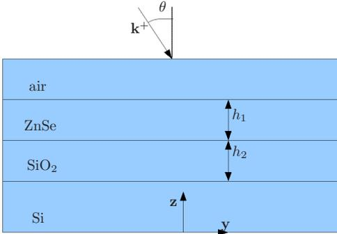
FIGURE 2. Schematic and notations of the slab under study.
