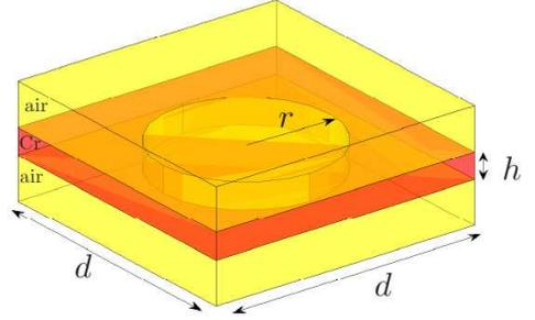
FIGURE 13. Schematic of the hole array under study.
