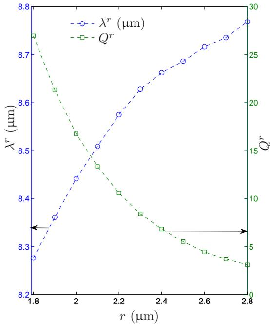
FIGURE 12. Resonance features  $\lambda^r$  and  $Q^r$  as a function of the hole radius  $r$ .
