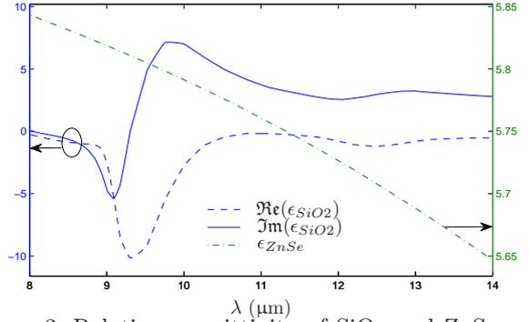
FIGURE 3. Relative permittivity of  $\text{SiO}_2$  and  $\text{ZnSe}$  as a function of the wavelength  $\lambda$ .
