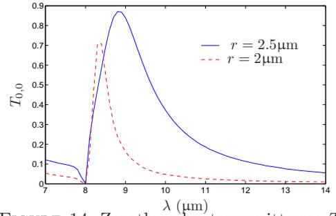
FIGURE 14. Zeroth-order transmittance  $T_{0,0}$  as a function of the wavelength for  $r = 2 \mu\text{m}$  and  $r = 2.5 \mu\text{m}$ .
