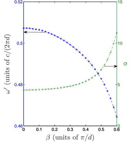
FIGURE 11. Lowest eigenfrequency and associated quality factor as a function of  $\beta$ .
