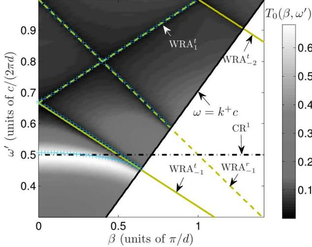
FIGURE 10. Colormap : zeroth-order transmittance  $T_0(\beta, \omega')$ ; + : dispersion diagram  $\omega'(\beta)$ ; — :  $n^{th}$  order Wood-Rayleigh anomalies in transmission  $WRA_n^t$  (solid) and reflection  $WRA_n^r$  (dashed); ·-·- : cavity resonance  $CR^1$ .
