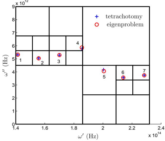
FIGURE 4. Loci of the resonance frequencies in the complex plane for the two methods.
