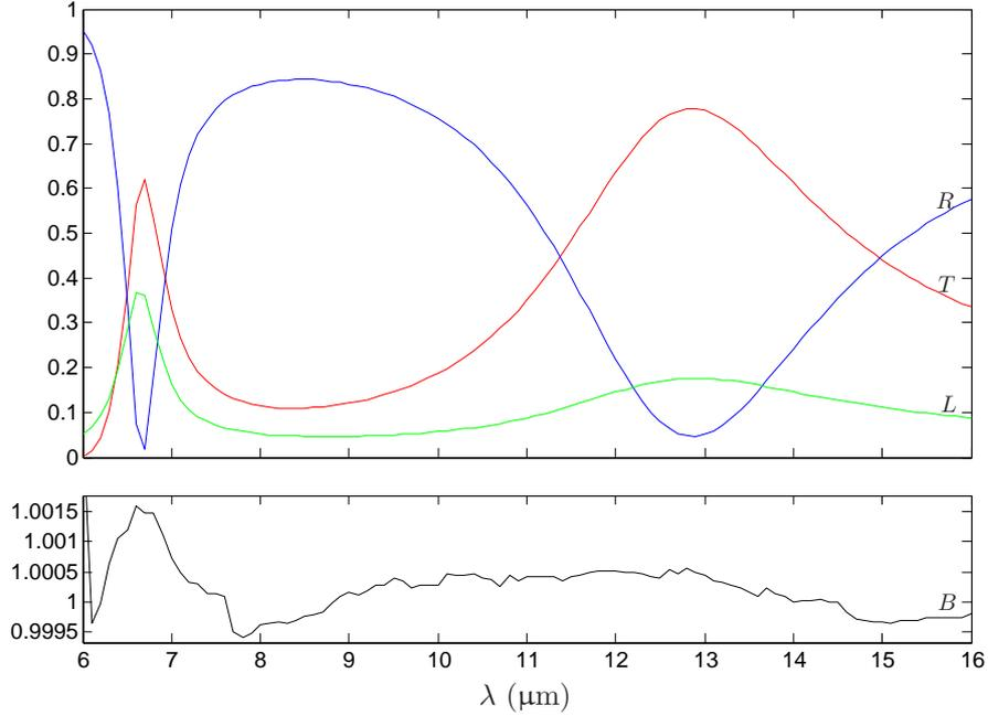
FIGURE 9. Zeroth-order transmission  $T$ , zeroth-order reflection  $R$ , Joule loss  $L$  and energy balance  $B$  as a function of the wavelength  $\lambda$ .
