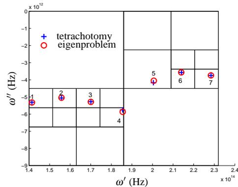
**FIGURE 3.** Loci of the resonance frequencies in the complex plane for the two methods.
