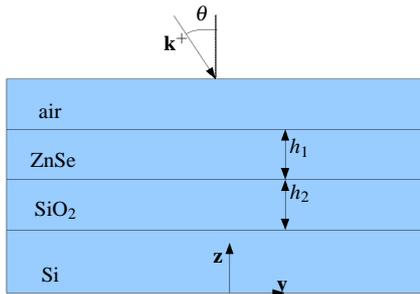
**FIGURE 1.** The multilayered slab under study.
