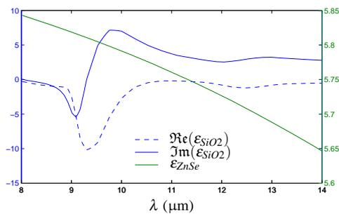
**FIGURE 2.** Relative permittivity of  $\text{SiO}_2$  and  $\text{ZnSe}$  as a function of the wavelength  $\lambda$ .
