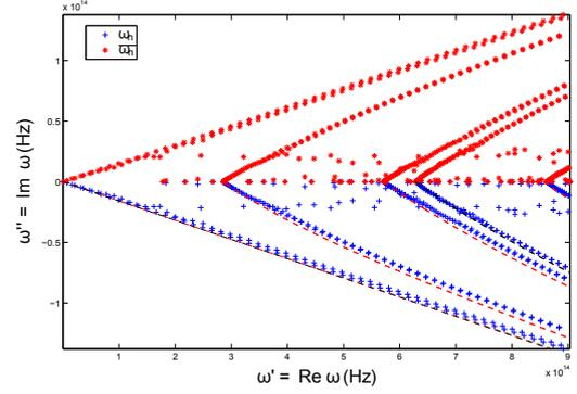
**FIGURE 2.** Quasi-modes of a grating with PML: “leaky modes” (individual +), essential spectrum (dashed lines) and its discrete numerical approximation (+ closed to dashed lines), and their complex conjugates (\* in upper half plane).
