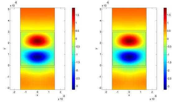
**FIGURE 3.** The scattered field computed using the modal method with 500 eigenvalues (left) is compared with the direct computation of the scattering problem (right). The maximum discrepancy is locally of the order of a few percent.
