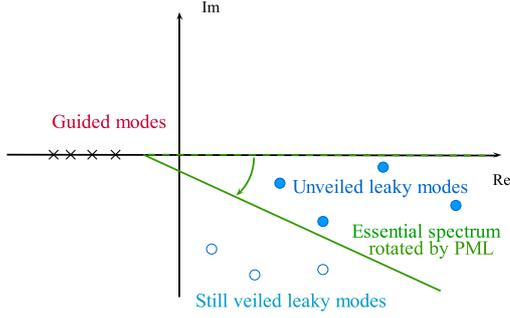
**FIGURE 1.** Guided modes, essential spectrum and leaky modes in an open waveguide.
